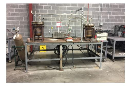
In addition, CEI has developed a dedicated system for the testing and calibration of a variety of alkalimetal-containing equipment (see photo above). Experimentally-confirmed operating curves for each flow meter can be derived with this apparatus, if necessary.
