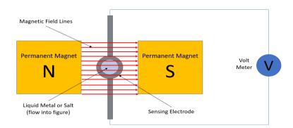
A liquid metal flowmeter is made by placing a nonmagnetic tube, such as stainless steel, between two faces of permanent magnets. The liquid metal acts as a moving conductor through the magnetic field. Electrodes are welded to the tube at right angles to the flow and the magnetic field to maximize the electromotive force (emf) sensed. The electrodes are of the same material as the tube to negate any galvanic response.
